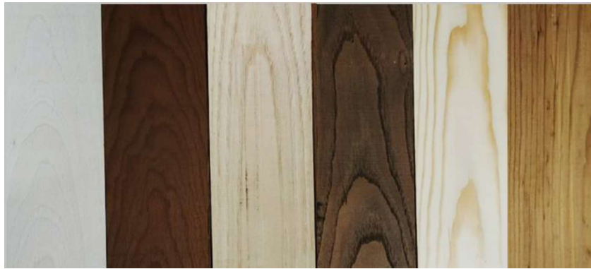
Figure 2 – Samples of control and heat-treated wood of beech, chestnut and Calabrian pine, from left to right.
