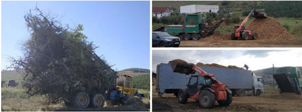
Figure 2 - A loaded forwarder on the left; the telehandler loading woodchips into the lorry on the right.
