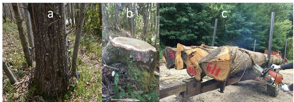
Fig. 1 In situ acoustic tomography test on a standing tree (a) and successive harvesting phase (b) and collection of a wood disc (c)
