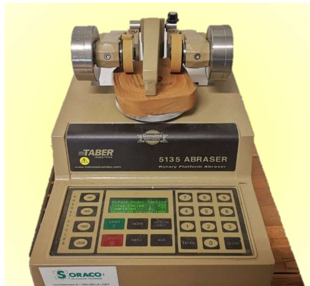
Figure 5 - Taber 5135 Rotary Platform Abraser during the abrasion test on a heat-treated Calabrian pine wood specimen.
