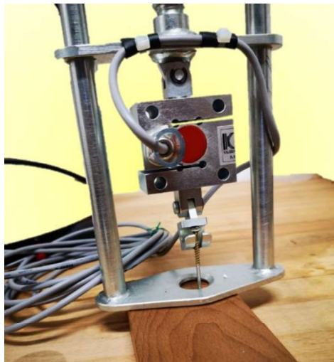
Figure 4 - SWRM device (Fakopp Enterprise Bt.) removing a screw of diameter 3 mm from heat-treated beech wood.
