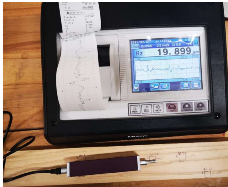
Figure 3. Surface roughness test by means the Mitutoyo SurfTest SJ-310.
