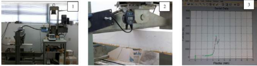
Figure 1. Universal bench for mechanical test with test specimen in flexion zone (1). Detail of the micrometer positioning and appearance of the first crack (2). Data extraction with MATLAB and break curve N-mm (3).
