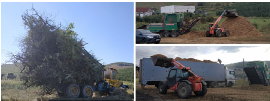
Fig. 2 A loaded forwarder on the left; the telehandler loading woodchips into the lorry on the right
