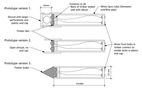
Figure 3. Prototype timber block probes [37].
