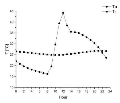
Figure 5. Average hourly exterior wall surface temperature for the entire period [46].
