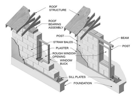
Figure 1. Load bearing (left) and post and beam with straw bale infill (right) [20].
