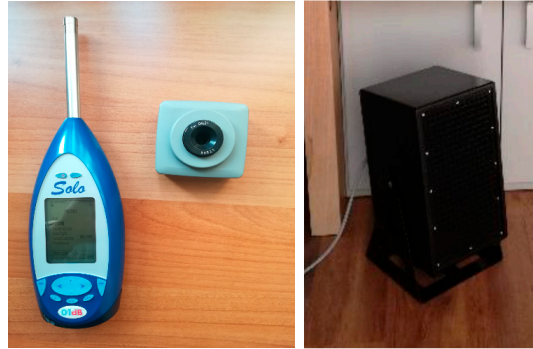
Figure 5. Left: Sound level meter Solo 01-dB with its condenser microphone and the calibrator Cal 21. Right: Directional loudspeaker.
