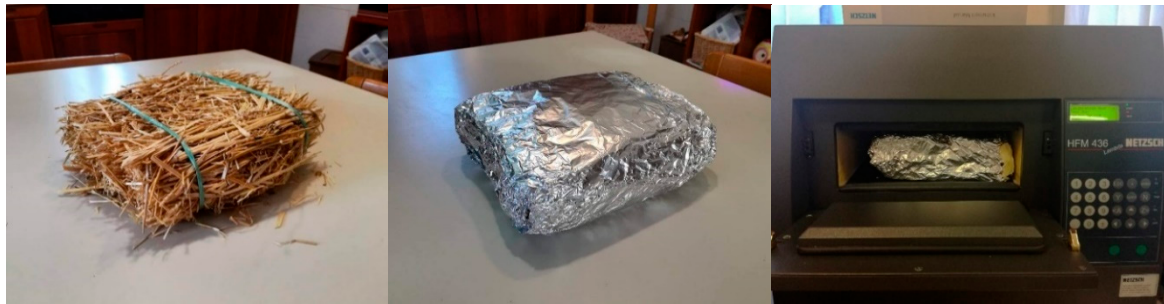
Figure 4. Specimen preparation and placement into the heat flow meter.
