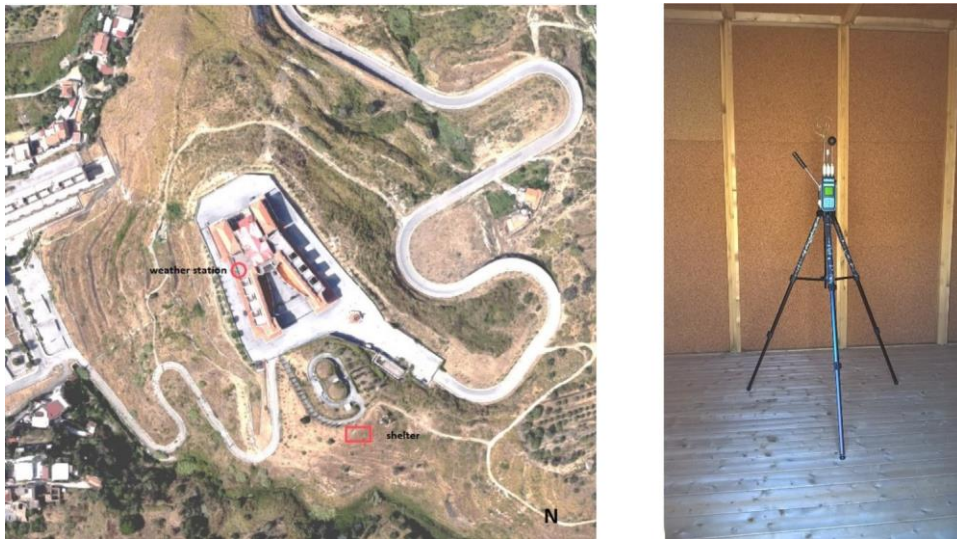
Fig. 7. Site of weather measurements at the University of Reggio Calabria and environmental sensor system inside the shelter prototype.
