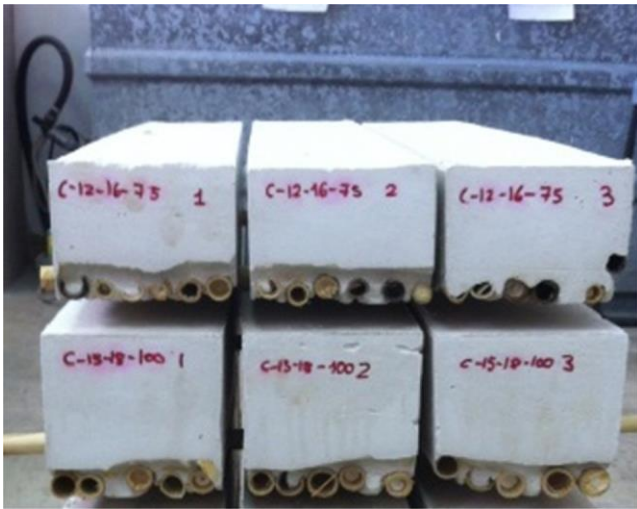
Fig. 6. Specimen series with 100 and 75 mm thickness in real size.
