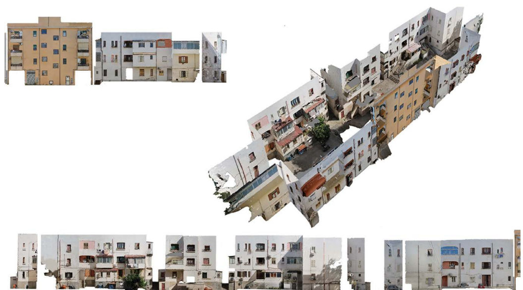
Fig. 2. Photogrammetric survey of block 80 of the Tremulini neighborhood of Reggio Calabria. Elaboration by Natale Mancuso.
