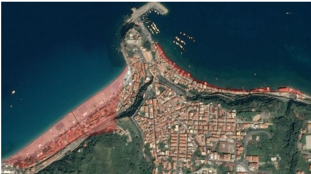
Fig 5.4 Inundation hypothesis in pink of 200 m near Livorno river and of 90 m along St. Nicola's Church in Marina Grande and of 10 m in Chianalea, (Bing, present day).
