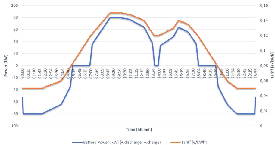
Figure 28. Dynamic electricity price and EMS scheduling in MATLAB/Simulink® over a 24-hour horizon, compressed into 24 seconds of simulation time, derived from realistic daily market tariffs in Italy: tariff profile vs battery charge/discharge scheduling under low/high tariffs.
