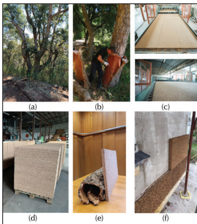
Figure 1 - Cork board production process: (a) Forests, natural origin of cork cycle; (b) Cork de-barking; (c-d) Ecological organic natural cork boards/panels production; (e) Cork: raw bark and board/panel for Green Buildings; (f) Ecological cork boards/panels make the Building: Green and Healthy. Source: Authors.
