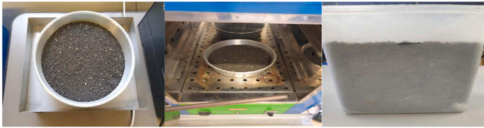
Fig. 1. Ash volcanic sample preparation to achieve the moist state.
