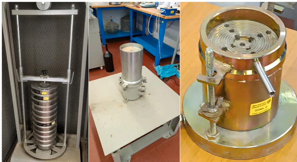
Fig. 5. Sieves for particle size analysis (on the left), maximum density equipment (in the middle), permeability test (on the right).
