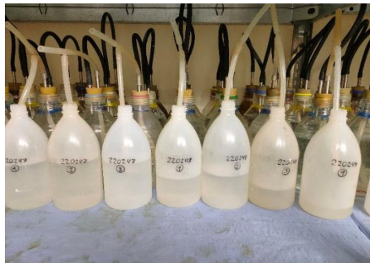
Figure 4.2 Reactors placed inside the climatic chamber at 37 °C.
