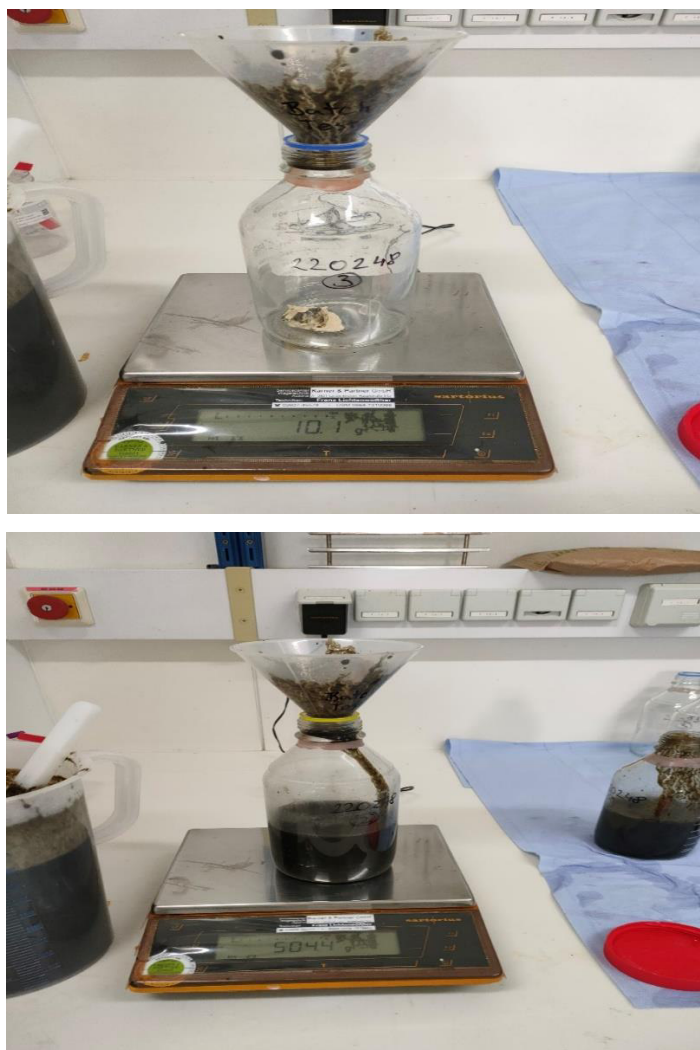
Figure 3.10 Weighing of samples directly into the reactors and addition of inoculum.
