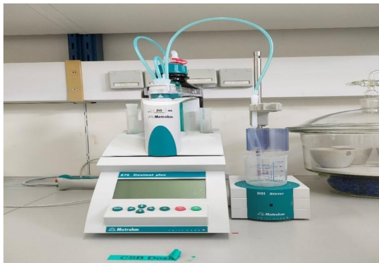
Figure 3.6 Metrohm 87G Dosimat plus used for sample titration.
