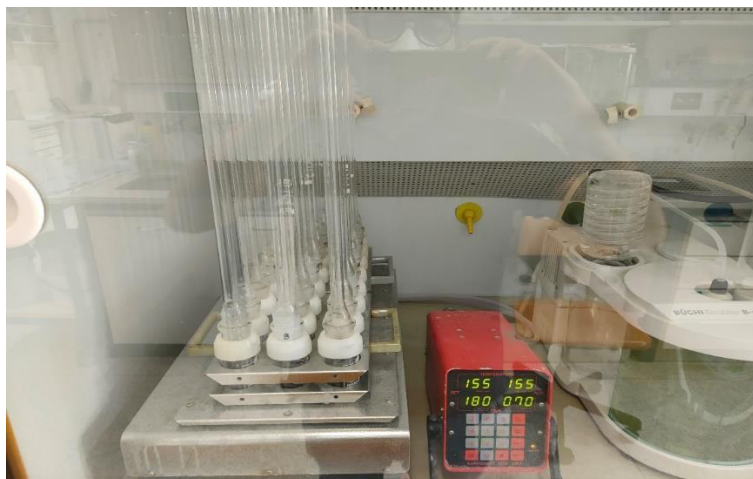
Figure 3.4 Samples thermally cycled 180 minutes at 150°C.
