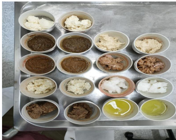
Figure 3.1 Fresh samples to be dried at 105°C.
