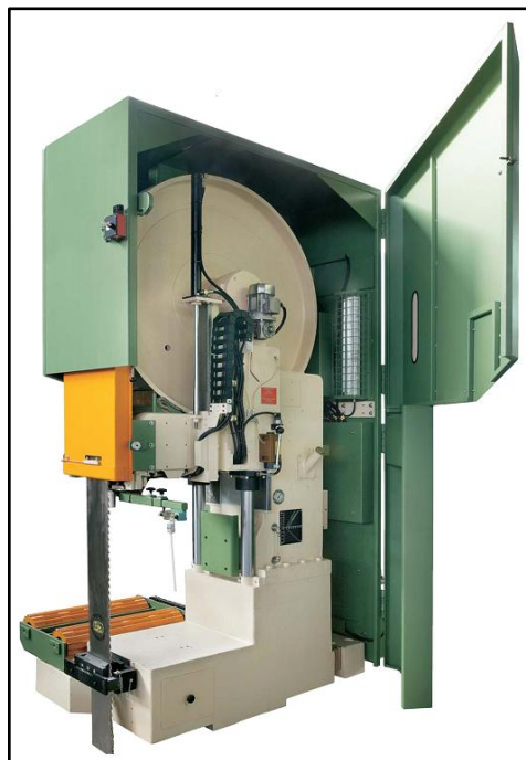
Figure 51. Hydraulic vertical log band saw
