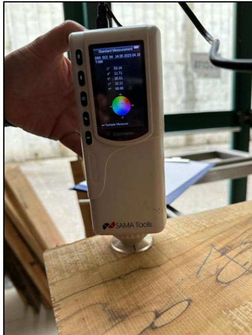
Figure 41. Color measurements with a SAMA tools colorimeter
