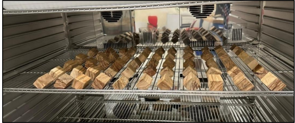
Figure 42. Specimens placed in a climatic chamber
