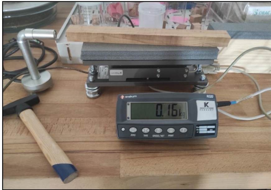
Figure 33. Specimens were tested by Portable lumber grader
