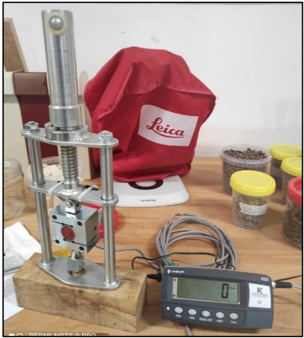
Figure 39. Specimens were tested by Screw Withdrawal Force Meter device
