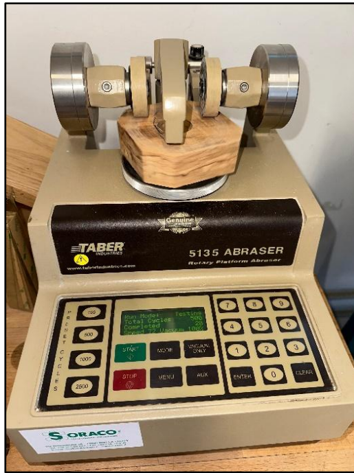
Figure 50. Abrasion test by Abrasimeter taber
