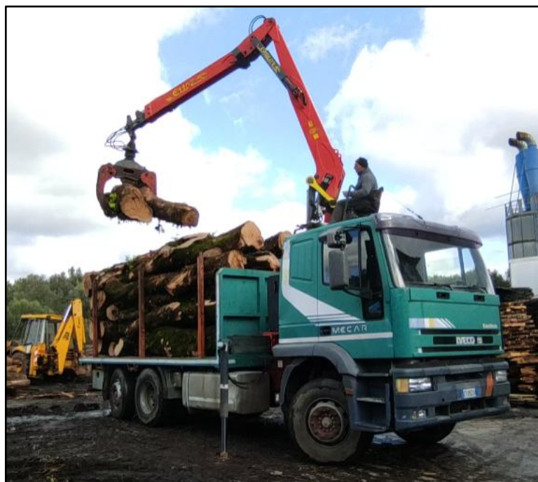
Figure 11. Truck equipped with a crane for transporting the logs.
