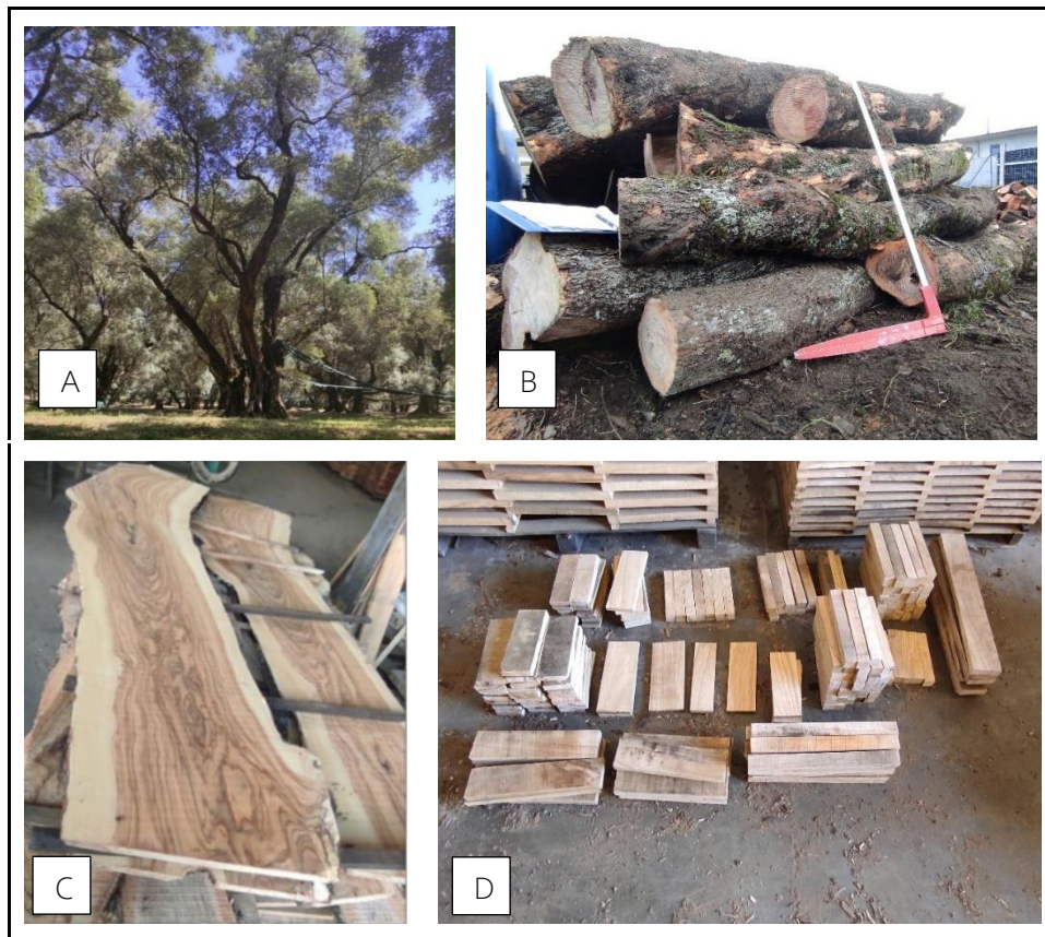
Figure 29. 'Sinopolese' olive trees (A), branches logs (B), branches sawn wood (C) and branches wood specimens for laboratory tests (D)
