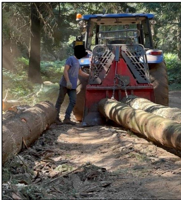
Figure 12. Timber extraction, with farm tractor equipped with forestry winch
