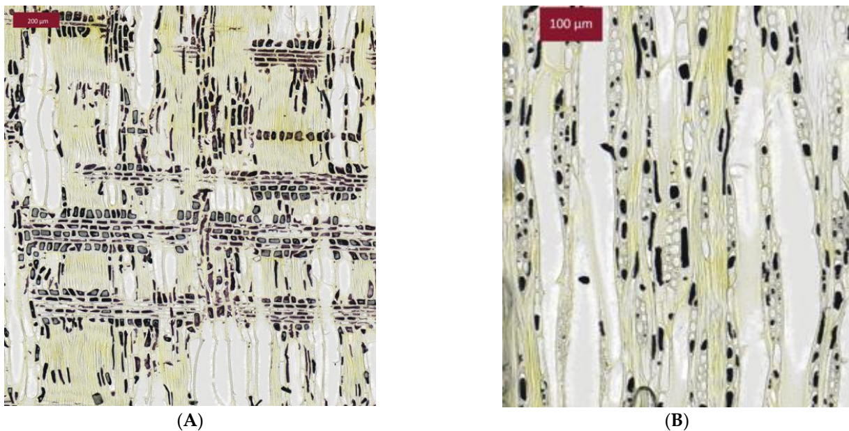
Figure 10. Starch (black spots) in Ottobratica olive wood cultivar, 5A sample, sapwood. (A) Radial section, (B) tangential section.
