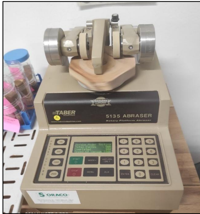
Figure 35. Specimens were tested by Taber Rotary Abraser 5135
