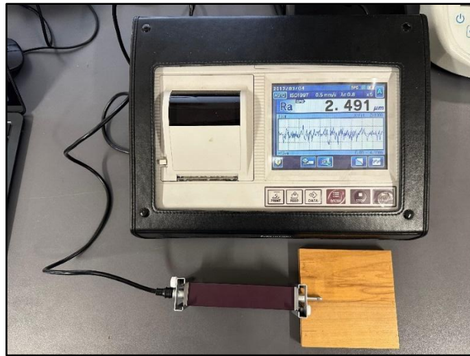
Figure 31. Roughness profile was recorded with a Mitutoyo SurfTest SJ-301
