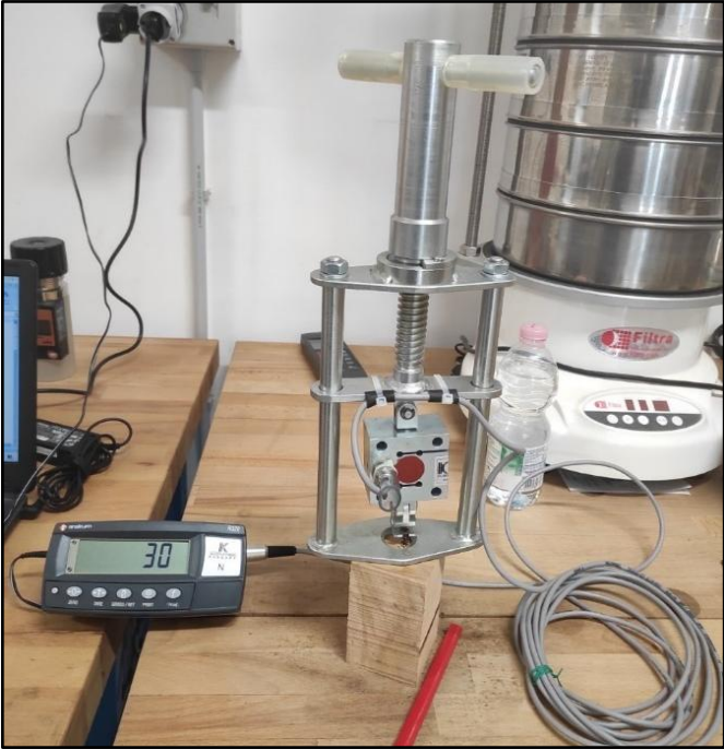
Figure 40. Specimens were tested by Screw Withdrawal Force Meter device
