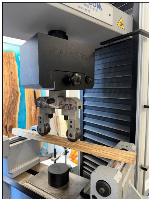
Figure 46. Test for determination of MOEs and MOR by four-point test.
