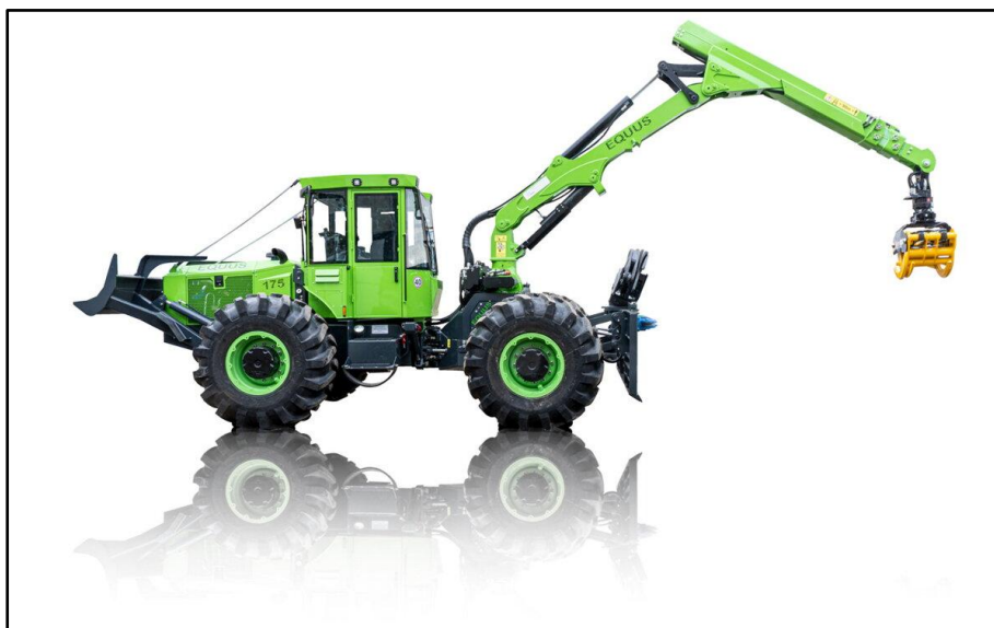
Figure 24. Equus 175 N skidder
