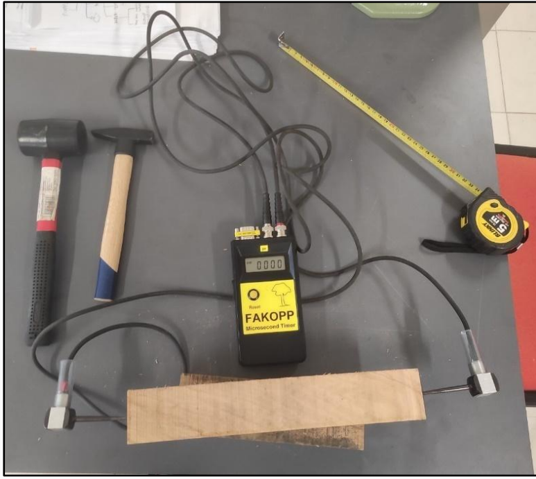
Figure 32. Specimens were tested by Microsecond Timer
