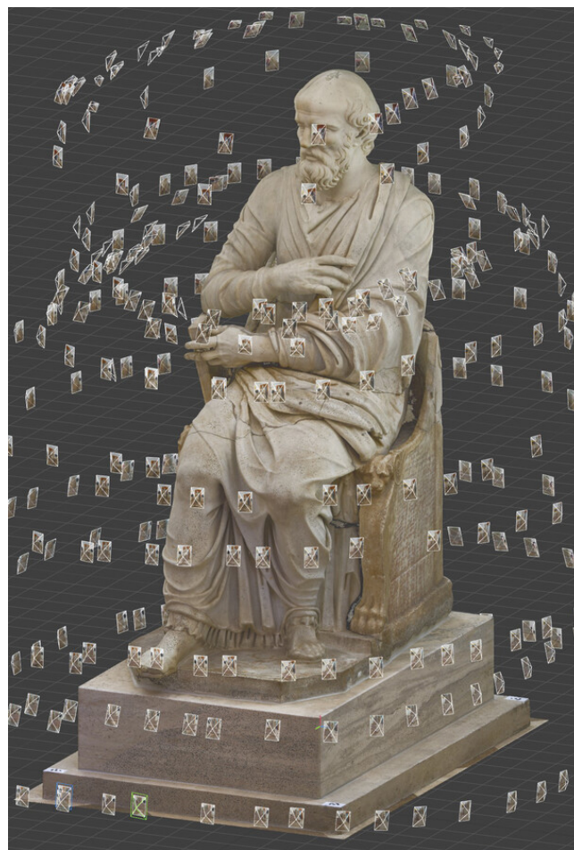
FIGURE 3 Visualization of the absolute positioning and orientation of the 419 shots used for the realization of the 3D model
