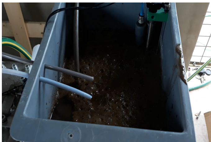
Figure 12. Distribution of sludge structure during ultrasonic treatment. A gradual disintegration of the agglomerates and a reduction in viscosity are observed, indicative of the cavitation effect induced by sonification, which facilitates the breaking of the particles and the release of intracellular and extracellular materials.
