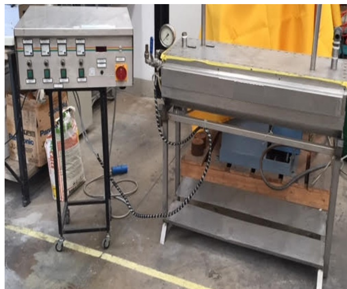
Figure 3. The experimental apparatus for sludge treatment process by ultrasonic sonication. Left: the amplifying device with current values increasing in percentage from 0 to 60 A. Right: the tank containing the sludge during ultrasonic sonication.
