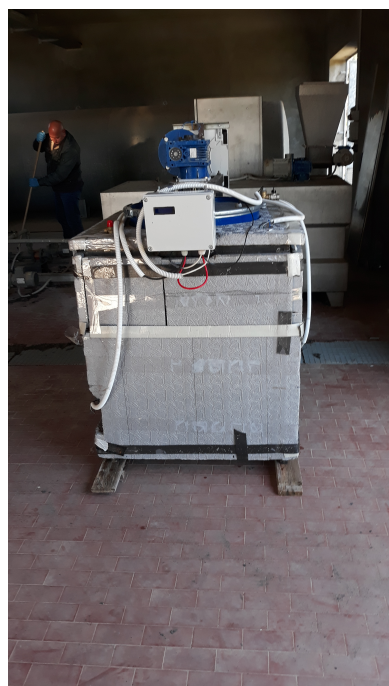
Figure 14. Prototype of a sludge mixing tank. Sludge, once sonicated, is deposited in a conveyor belt and fed into the prototype. Equipped with a temperature sensor and a humidity sensor, the prototype mixing tank heats the already ultrasonically treated sludge, further reducing the amount of water and consequently making it lighter.
