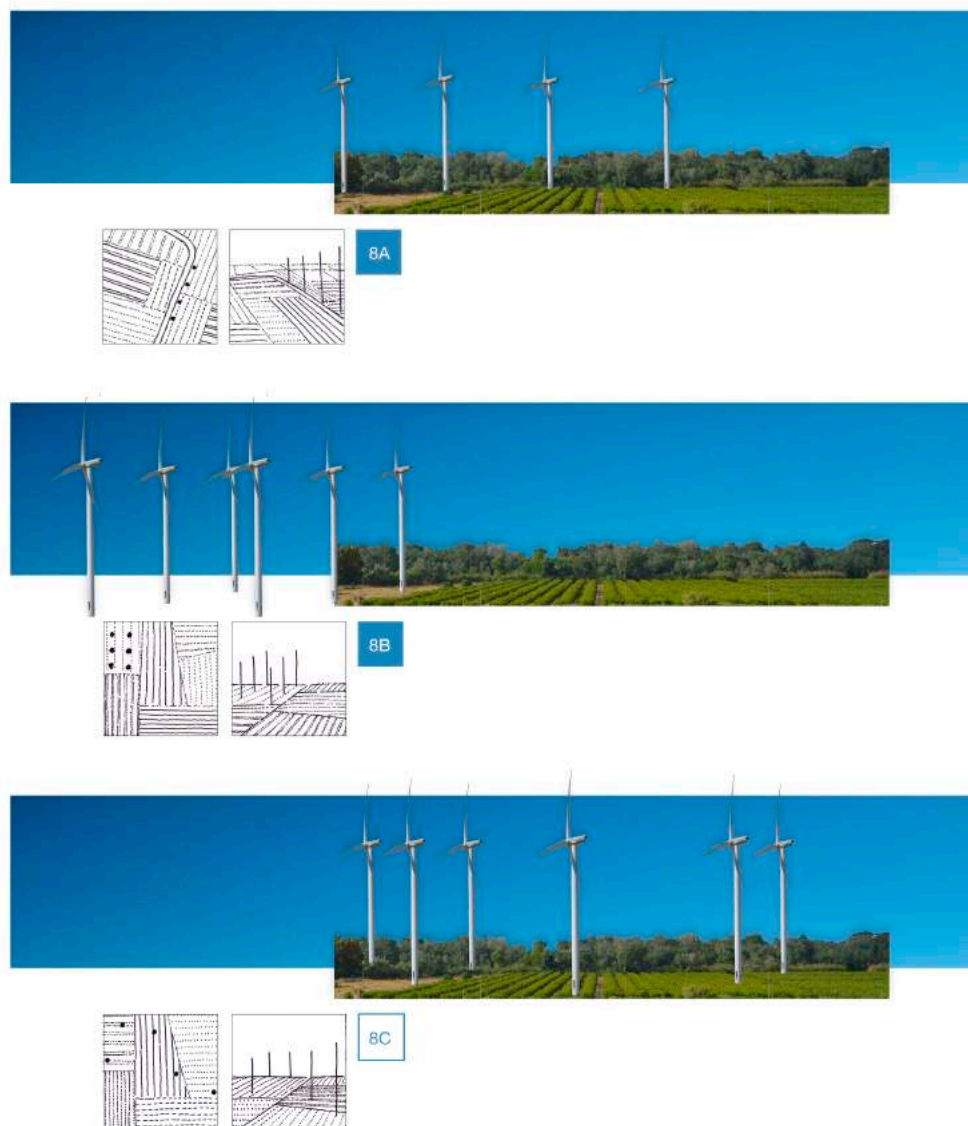
Figure 3. Agricultural structures. Examples of criteria. 8A. In agricultural landscapes with well-defined traces (plots, paths, canals, fences, tree alignments, dry stone walls, etc.), a linear arrangement following these traces favors good insertion in the landscape and facilitates its reading. 8B. Geometric arrangements with clearly perceptible rhythms and layout patterns (within the same plot or set of regular plots), and with appropriate wind turbine heights, can generate good integration into the site. 8C. A wind development that does not follow the layout of the agricultural landscape expands the sense of disorder and distortion of the scene. (All images and photo-simulations in this article were taken from the document “Wind Energy and Landscape. Guidelines for a suitable installation in Catalonia”. They were drawn up by the research group).
