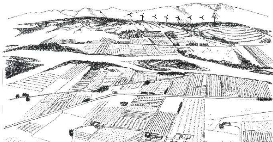
Figure 6. River terraces 1.2. Example of installation hypothesis in a representative scenario through the application of the identified criteria. Criteria adopted: 2: In general, wind turbines are arranged according to clear and regular geometric organizations (lines, curves, grids, etc.) and from the landscape patterns of the place to provide readability to the whole and reduce the feeling of clutter and visual confusion. 4: Spacing is regular between wind turbines and wind turbines of the same model, height, and color are used to emphasize the order and consistency of the set. 1A: In the presence of successive reliefs, the location of the wind turbines in intermediate saws reinforces the perception of a greater depth of field and a greater understanding of the scenario. However, prioritizing compact implements of linear composition avoids fragmentation and dissemination and ensures readability of the whole. 3A: The linear arrangement of wind turbines in a wavy landscape following their morphological characteristics generates a clear and balanced image. 5B: It is important that the location and size of the wind turbines are consistent with the overall scenario and do not compromise the differentiated characteristics of the mountain and lowland agriculture. 9B: Locating several wind turbines next to the town center or an urbanization, as long as it is measured and ordered and far enough away, can create new points of attraction, but without distorting the perception of the whole. B: The implementation hypotheses offer indicative heights for wind turbines starting from 50 m. (All images and photo-simulations in this article were obtained from the document “Wind Energy and Landscape. Guidelines for a suitable installation in Catalonia”. They were drawn up by the research group).
