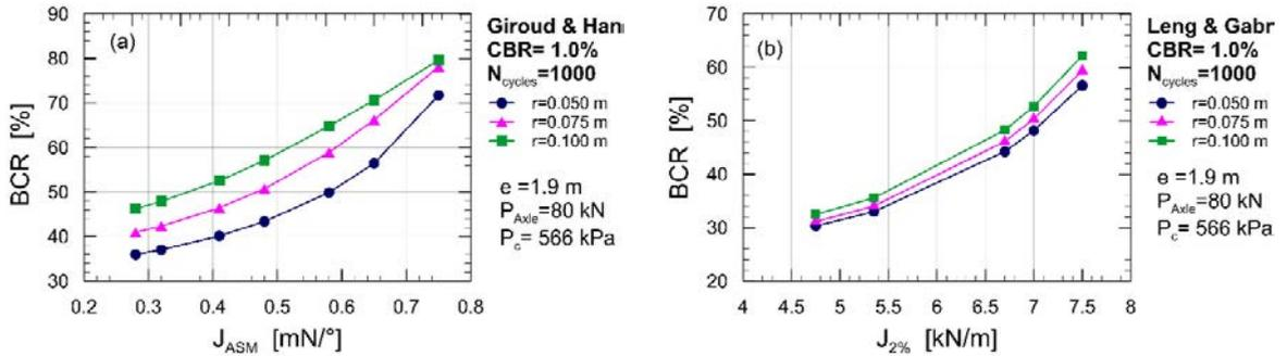
Fig. 2. Unpaved roads design procedures - Iso-rutting curves relating to Base Course Reduction factor (BCR) at  $N_{cycles} = 1000$  and varying reinforcement stiffness (for mechanical parameters relating to geosynthetic mechanical properties see Calvarano et al. [19] : a) Giroud et Han [3, 17]; b) Leng and Gabr [18].
