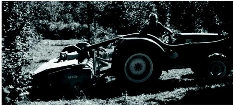
**Figure 1.** Hazelnut mechanical harvesting from the ground using the Jolly 2800 machine.
