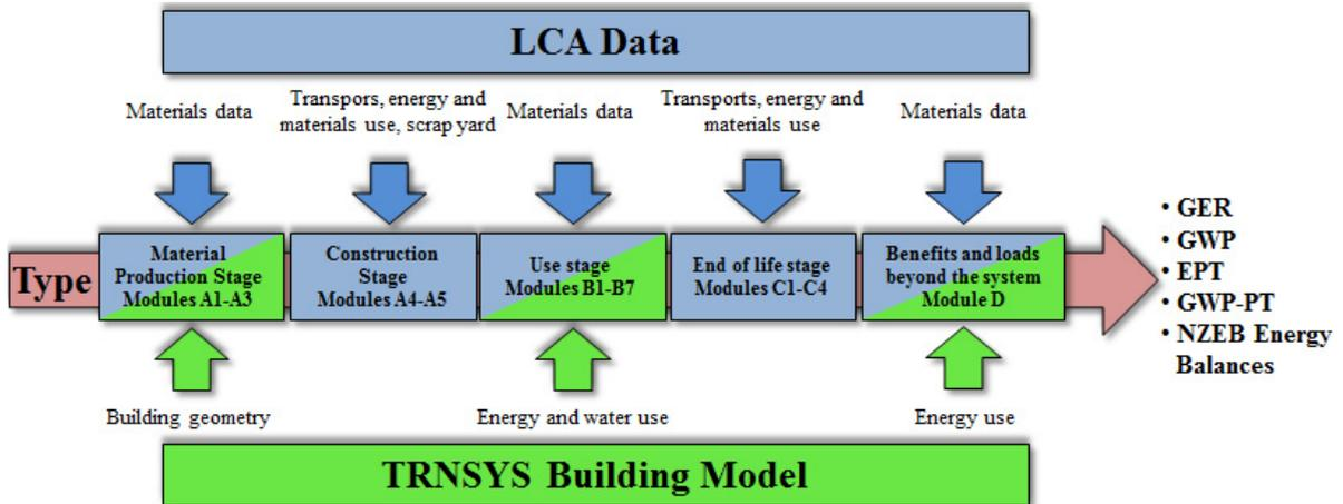
Fig. 1. Schematic description of the TRNSYS Type.
